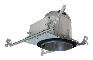
To supply and install Tamlite DL6MED Series of line voltage recessed fixtures as specified. The fixture shall operate at 120VAC. Lamps shall be as specified, medium base lamps up to a maximum of the rated lamp wattage on the fixture nameplate. The lamps shall not be supplied with the fixture. The fixture shall be c-UL-us approved.
